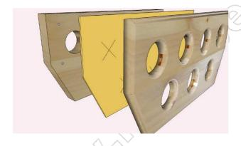
I designed the rubber sheet in yellow to make clear the cuts (which were not visible on black background). I had at my disposal a rubber sheet of about 1.5 mm thick I think a piece of inner tube truck recovered from a tire dealer could very well agree.
